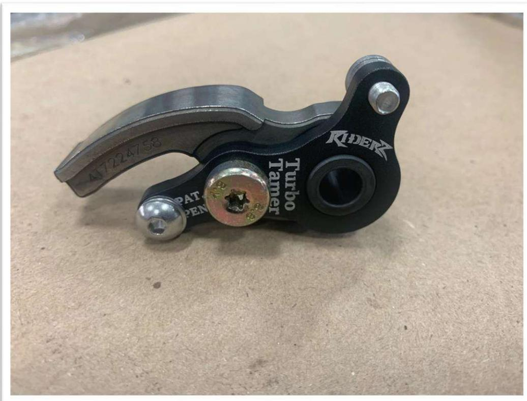
Ramp with Turbo Tamers installed.
